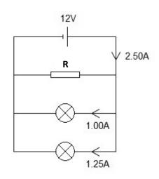
Calculate the power dissipated by resistor **R**.
