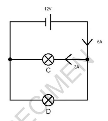
Use the formula **resistance = potential difference ÷ current** to calculate the resistance of
