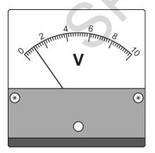
Name the error on the voltmeter and suggest how it should be dealt with.
